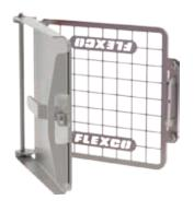
Chute Opening: 600 mm x 600 mm Outer Door: Solid c/w Lockable Handle Inner Mesh Door: 3 mm mesh @ 50 mm spacing Material: Grade 316 Stainless Steel Overall Weight: 32 kg
