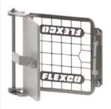
Chute Opening: 500 mm x 500 mm Outer Door: Solid c/w Lockable Handle Inner Mesh Door: 3 mm mesh @ 50 mm spacing Material: Grade 316 Stainless Steel Overall Weight: 18 kg
